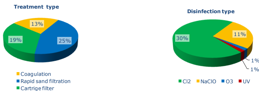
Figure 3.8: Treatment of pool and spa water applied in hotels.
